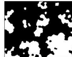
An open-close Alternating Sequence Filter (ASF) removes salt-and-pepper noise. Each successive iteration removes particles of a larger diameter. One, five, and fifteen iterations are shown.
